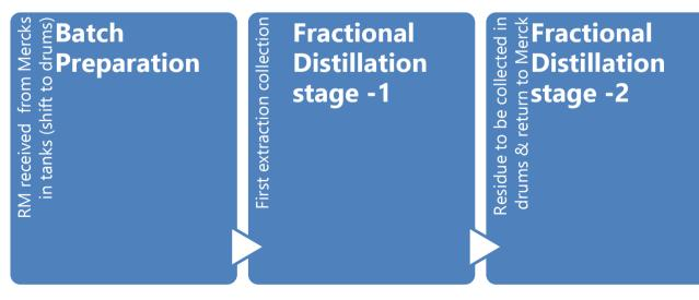
Figure 4.1: Production process of Solvent Distillation
