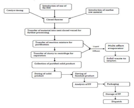
Figure 4.2: Prodction process of Anti-oxidant
